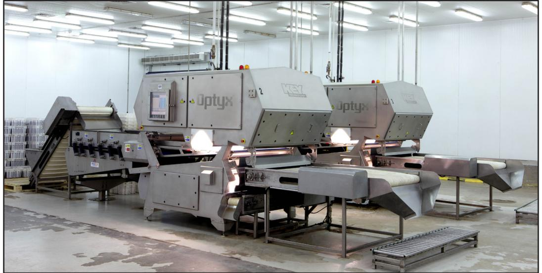
Using cameras, Optyx recognizes each object's size and shape as well as millions of subtle color differences. AI Foah uses this capability to grade dates according to size and color. Lasers detect foreign material (FM) based on differences in the structural properties of the objects, a capability that AI Foah uses to remove dates with calyx when they are producing the highest product quality for the Abu Dhabi royal family.
