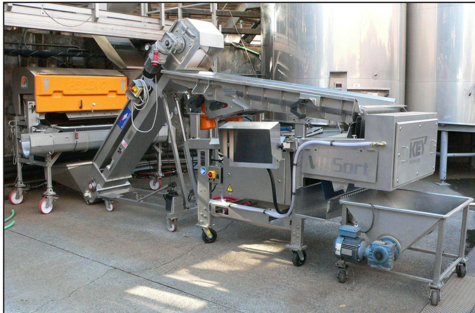
The stainless steel VitiSort is compact and mobile, designed to easily roll into position under the destemmer so fruit automatically flows from one machine to the other.
