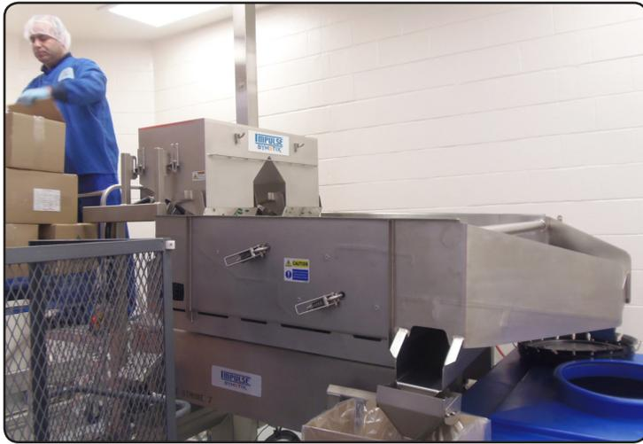
deck removes broken tablets and fragments, and the lower deck recovers usable tablets, which helps keep nuisance rejects – the loss of good tablets – to a very low and acceptable volume.”
