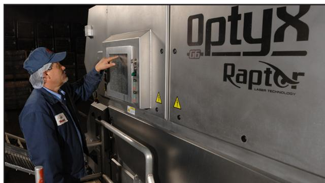
Optyx with Raptor is a versatile platform that can be configured for either single-side or top-and-bottom scanning by multiple sensors including color, Vis/IR (visible infrared), and monochromatic cameras as well as Raptor Laser Technology and Key's newest FluoRaptor™ fluorescence-sensing laser technology. To
