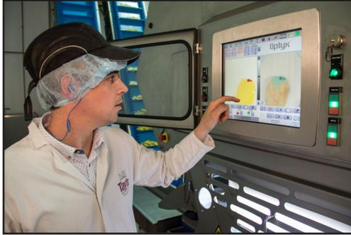
Tayto operates most of their production lines 24 hours a day, six days a week, with the seventh day spent cleaning. “Optyx is well designed for sanitation,” said Hoden. “It takes one person a couple of minutes to remove the belt, which is then washed. The rest of the machine is wiped down. It’s all very easy.”
