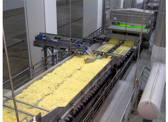
Even when incoming product quality is good, ADRFirst can improve yields. Since 1999, ADR systems have featured multispectral cameras that enable object recognition, allowing the system to identify individual strips. In addition to cutting defects, ADR can make a wide range of smart cutting decisions that help processors get the most from their product.
