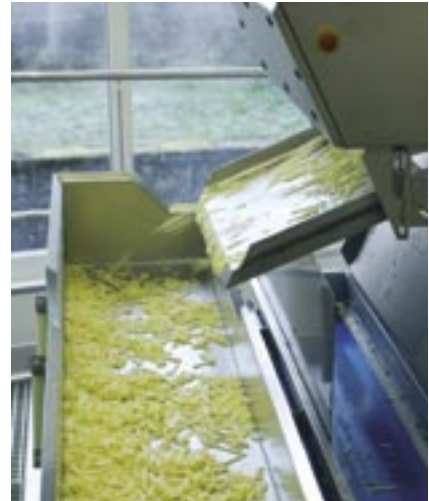
Discharge from Optyx on shredded potato line
