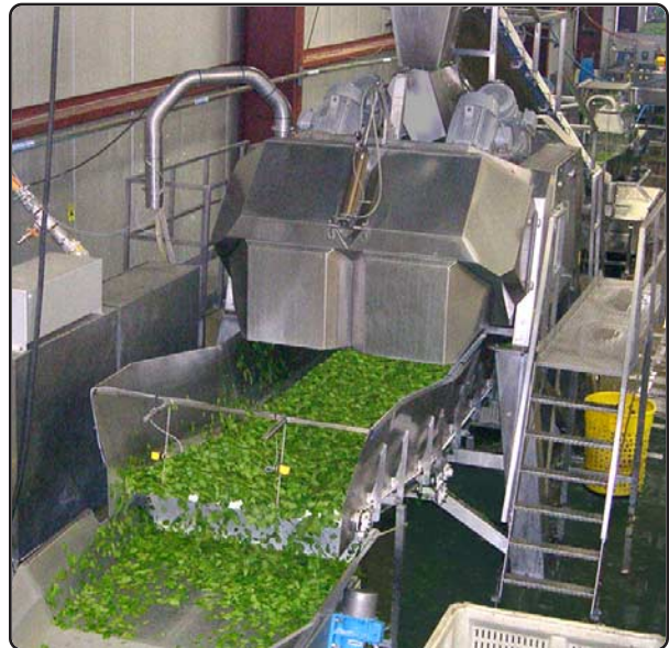
Key's four-drum automatic dryer provides a continuous flow of dried tender leaf, maximizing volume and minimizing damage
