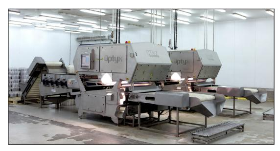
Using cameras, Optyx recognizes each object's size and shape as well as millions of subtle color differences. Al Foah uses this capability to grade dates according to size and color. Lasers detect foreign material (FM) based on differences in the structural properties of the objects, a capability that Al Foah uses to remove dates with calyx when they are producing the highest product quality for the Abu Dhabi royal family.
