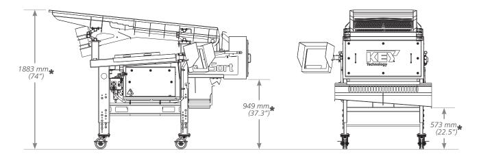
★ Vertical dimensions are adjustable from +406 mm to -152 mm (+16" to -6")
