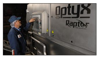
Optyx with Raptor is a versatile platform that can be configured for either single-side or topand-bottom scanning by multiple sensors including color, Vis/IR (visible infrared), and monochromatic cameras as well as Raptor Laser Technology and Key's newest FluoRaptor<sup>TM</sup> fluorescencesensing laser technology. To
