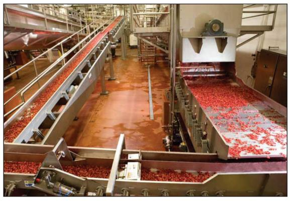
Iso-Flo vibratory shakers form an integral part of the sanitary Ocean Spray processing line.
