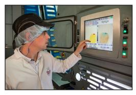
Tayto operates most of their production lines 24 hours a day, six days a week, with the seventh day spent cleaning. "Optyx is well designed for sanitation," said Hoden. "It takes one person a couple of minutes to remove the belt, which is then washed. The rest of the machine is wiped down. It's all very easy."
