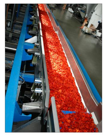
The Impulse shakers and Key weighing hoppers are integrated with the microwaves via a centralized controller. Each of Paula's snack products are stored in the system's memory, which automatically
