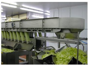
that combined will equal 100grams. Typically, the scale chooses between 3 to 5 buckets in combination. The computer on the scale is constantly looking at individual bucket weights in search of the perfect combination.
