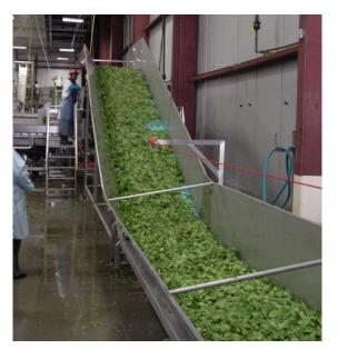
Although a total cost of ownership analysis indicates that vibratory and horizontal motion conveyors are less expensive than belt conveyors in the long run, there are applications that are best served with belt conveyors, warranting their use despite the higher cost.
