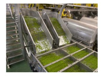
Electromagnetic shakers allow lower conveying pan amplitudes at higher frequencies to be varied, which make them ideal for lines that handle a wide variety of products or lines that require precise metering.
