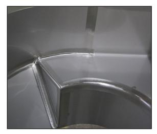
The most hygienic conveyors feature no enclosed hollow bodies that could harbor bacteria and leak. Hollow bodies such as tubes, which have traditionally been used on conveyor frames, are increasingly being replaced by open-section supports made of plate or formed sheet metal. Conveyors designed with free draining surfaces, with even the conveyor bed at enough of a slope to drain, minimize the build-up of moisture during production and eases washdown.
