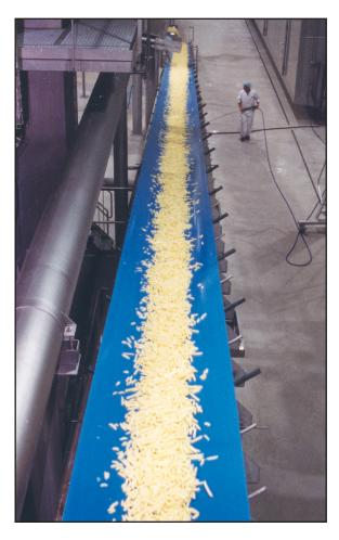
on sprockets like a modular plastic belt conveyor and are not under tension, which allows for easy lifting of the conveyor belt for relatively fast and thorough cleaning.
