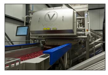
berries per hour. Key equipped Emblème's sorter with front- and rear-mounted laser scanners that operate within the visible light and near-infrared wavelengths. VERYX performs object-based sorting, recognizing both the colors of objects and their structural properties and selecting optimal ejection strategies for each item in the product stream.
