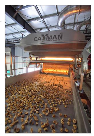
with very low false reject rates. This innovative sorter can easily handle high defect loads, including spikes of more than 50 percent, which makes it ideal for use after the cracker to separate shells from kernels.
