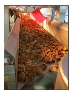
"This cascading line of three sorters is much more efficient than running three passes on one sorter. It's also much gentler. What hurts walnuts isn't flying through the air, it's accelerating and decelerating. Dropping into a bin or out of bin is what damages walnuts."
