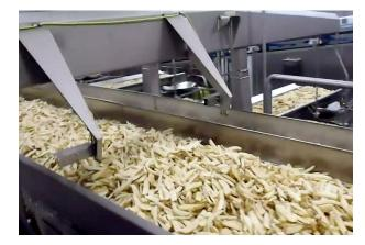
The distribution shaker can be a traditional vibratory shaker or a horizontal motion shaker. Horizontal motion shakers are ideal for many fragile, seasoned, coated, and frozen foods because they offer gentle, quiet, and sanitary conveying. Both conveyor types can be fitted with standard slide gates, flip gates, pivot gates, or proportional-control gates to discharge product to downstream equipment.
