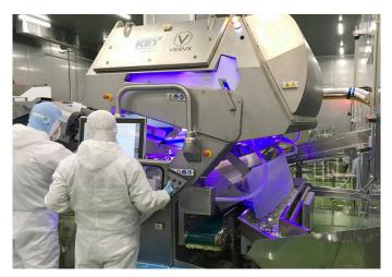
or air jets. Two-way sorters separate the stream into good product that makes grade and 'rejects' that include FM and defective products. Three-way sorters can be programmed to separate good product into two grades, while removing FM and defects into a reject stream.
