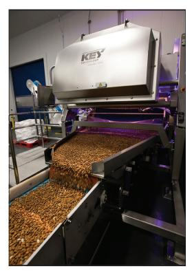
Pixel Fusion™ technology, producing a unique 'signature' for each material substance to detect the chemometric and biologic properties of objects. This versatile nut sorter finds and removes the widest variety of FM and even hard-to-detect defects like nuts with insect damage, rot and mold without false rejects, regardless of incoming defect loads, while also shape sorting and color grading.
