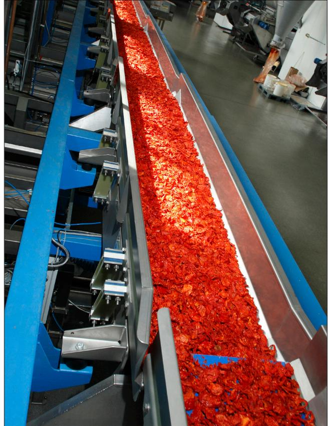
The Impulse shakers and Key weighing hoppers are integrated with the microwaves via a centralized controller. Each of Paula’s snack products are stored in the system’s memory, which automatically sets the shaker’s amplitude and the amount of product – from three to five kilograms – that the weighing hoppers accumulate and load into the microwaves during each cycle.
