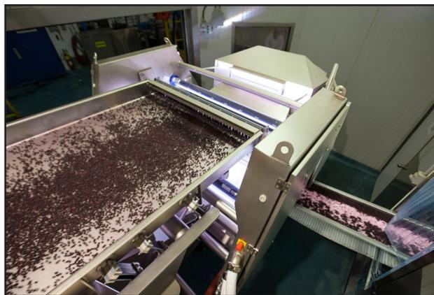
To sort up to nine metric tons of frozen berries per hour, Quebec Wild Blueberries selected the high-volume chute-fed VERYX C140, which features a 1400-mm wide inspection area. To maximize product quality, this sorter is equipped with front- and rear-mounted laser sensors and color cameras and Key’s advanced multi-sensor Pixel Fusion™.
