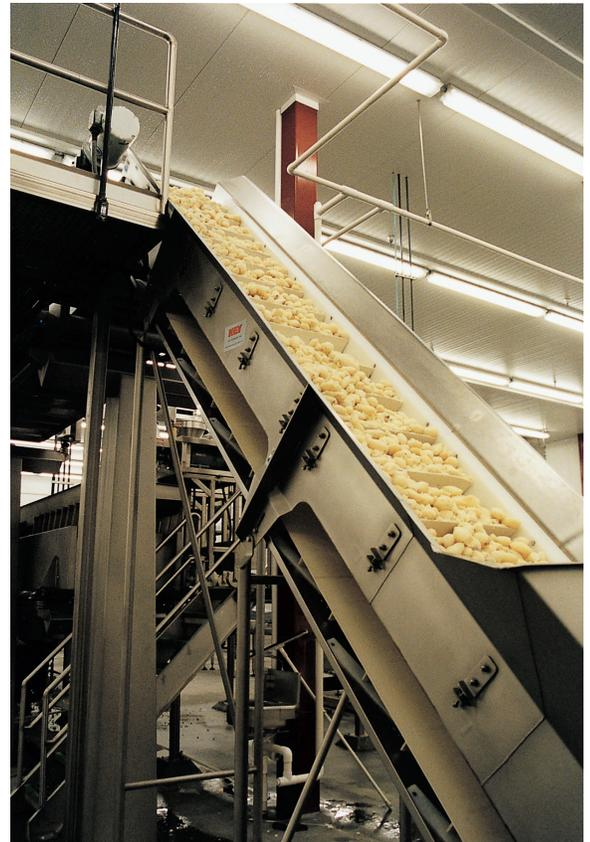
Although a total cost of ownership analysis indicates that vibratory and horizontal motion conveyors are less expensive than belt conveyors in the long run, there are food applications that are best served with belt conveyors, warranting their use despite the higher cost.
