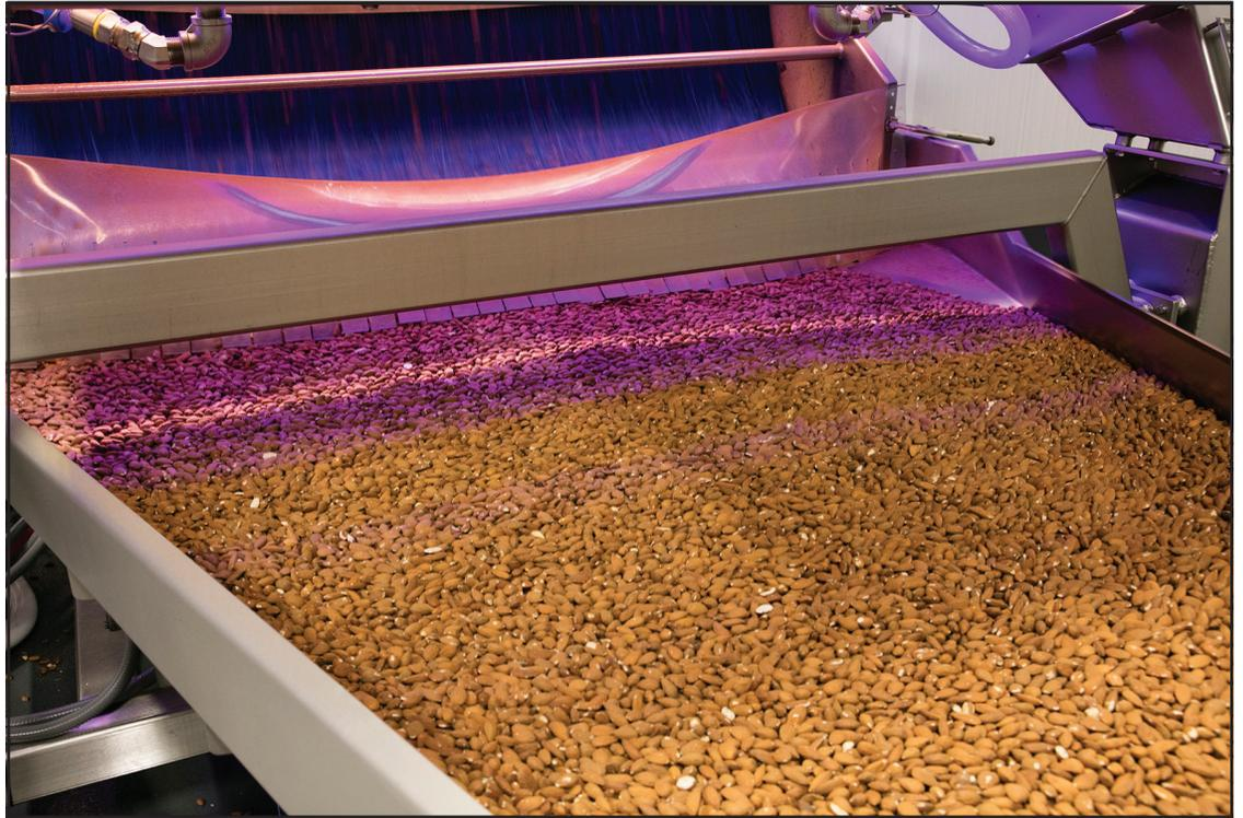
Caro Nut's VERYX BioPrint C140 features front- and rear-mounted hyperspectral sensors and high resolution color cameras. It can sort up to 8 metric tons of cashews, almonds, macadamia nuts and other nuts per hour.
