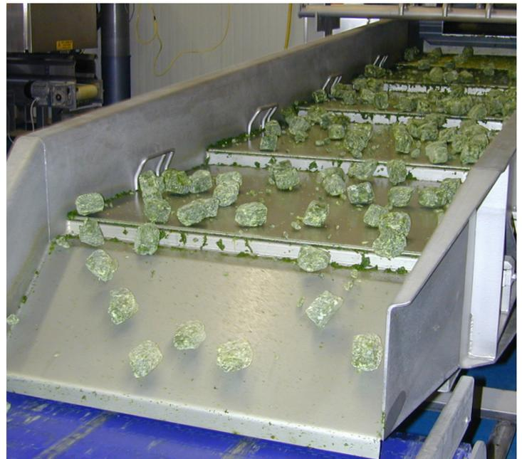
drives and horizontal motion conveyors can also be used effectively in many scale feed applications, depending on the product.
