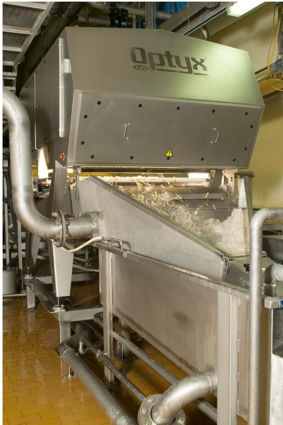
Strip-Length-Control is a subset of Sort-to-Grade that focuses on strip length. It is also dynamic in that it automatically preserves the length profile of final product despite the length of incoming strips fluctuating as the sizes of whole potatoes vary. This new sorter capability allows potato strip processors to eliminate mechanical length grading methods and the product damage they can cause.
