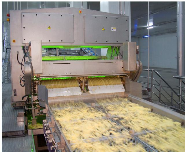
Sort-to-Grade is a powerful new capability that enables select sorters or automatic defect removal (ADR) systems to control the quality of output to a defined grade. By evaluating potato strips with minor defects against the current grade count, the sorter can allow some of those strips with minor defects to pass and still maintain grade. Tests show that Sort-to-Grade can increase yields by one to three percent while assuring final product quality.
