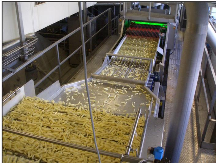
ADR 4 uses a belt conveyor, LED light source, Vis/IR (visible infrared) cameras, a patented rotary cutter with air-actuated knives, and Iso-Flo® vibratory conveyor to align, singulate, inspect, and trim defects from peeled and peel-on French fries and remove the defects from the product stream. Unlike traditional sorters, which remove the entire potato strip when defects are identified, ADR cuts the strip and removes only the defect.
