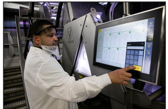
New automation intelligence helps maintain peak performance while easing use by allowing a sorter to run virtually unattended during normal production. In addition to STG, which makes the smartest accept/reject decisions to achieve grade and maximize yields while eliminating manual adjustments, today's most intelligent sorters offer a host of smart features.
