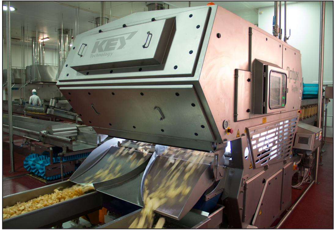
*Sanitation is of paramount importance throughout the process, so special attention must be exercised in equipment design, equipment transfers, proper speeds, proper strokes and proper arm angles. Also, equipment type must be appropriate for the application including various lofting vibratory conveyance systems, horizontal motion conveyance and elevating belt conveyor systems.*
