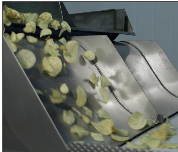
traditional belt conveyors to improve sanitation. This shaker features a wire mesh bottom and air knives overhead to remove the water and starch. Operating at a high speed and stroke, this system singulates chips and blows excess water off then feeds the fryer.
