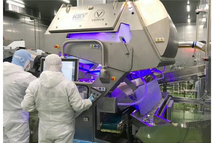
Although sorters are designed for continuous in-line product inspection at full production speeds, they can also be used in a batch-feed mode.
